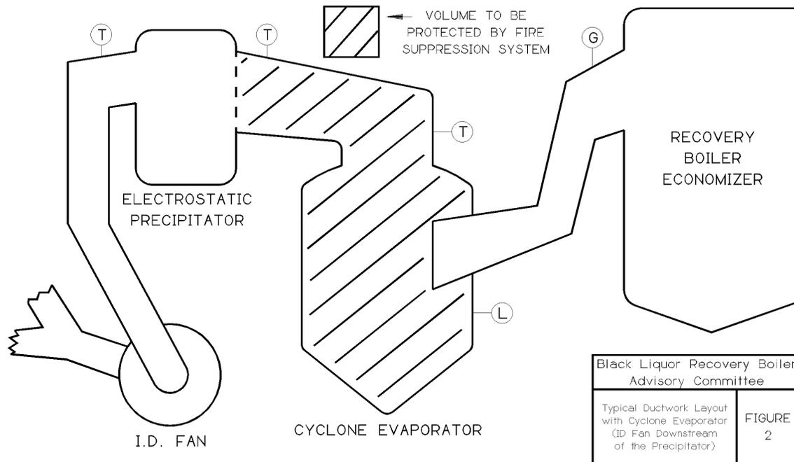
Fig. 2. Typical Ductwork Layout with Cyclone Evaporator (ID Fan Downstream of the Precipitator).
